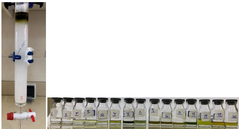
Fig. 3. Fractionation of coriander oleoresin by silica gel column chromatography and eluted fractions.
